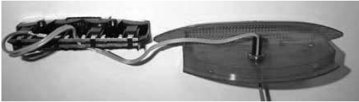
Fig 24 Wire routing through light unit
