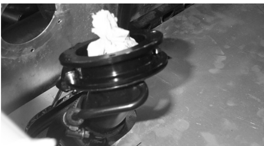
Fig 18 Spacer fitted to filler neck
