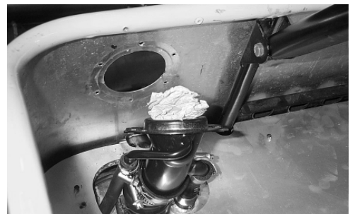
Fig 15 Old filler boss removed
