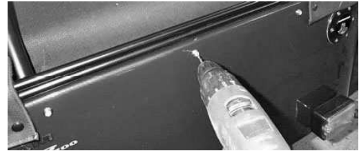
Fig 22 Drilling central popper on SV
