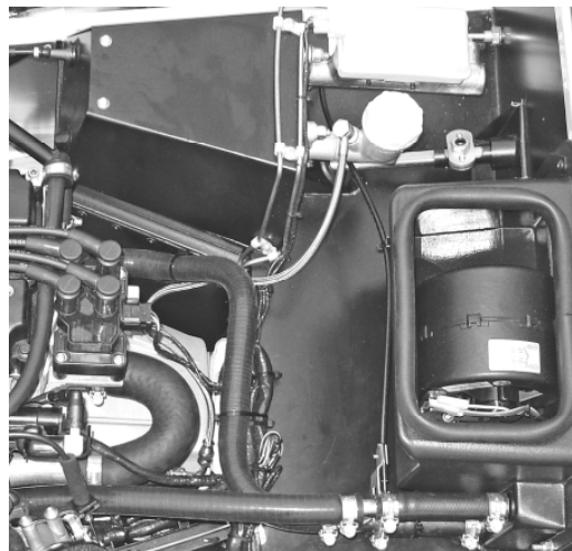
Fig 8 Clutch hydraulic hose
