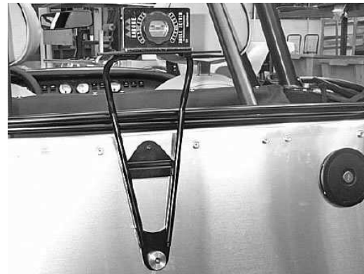
Fig 23 Alignment of bracket
