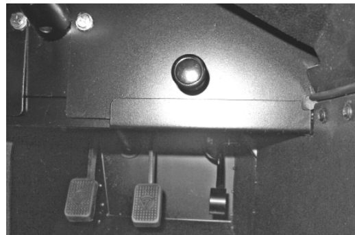
Fig 21 Heater control location
