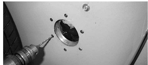
Fig 14 Drill out the six rivets
