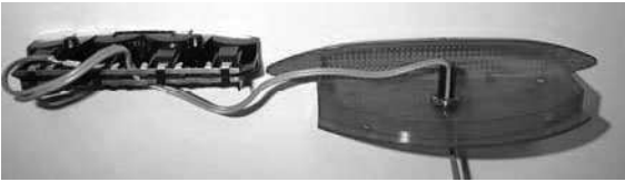
Fig 24 Wire routing through light unit
