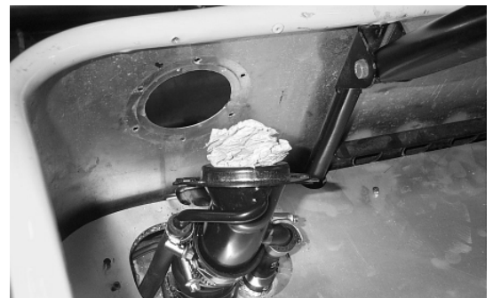
Fig 15 Old filler boss removed
