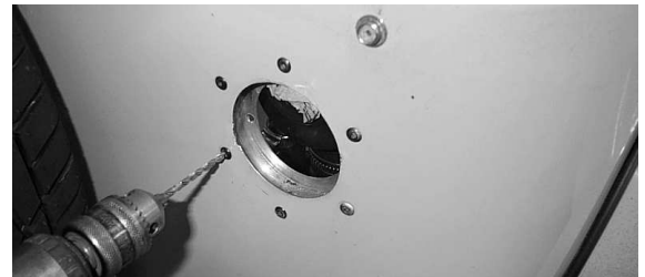
Fig 14 Drill out the six rivets
