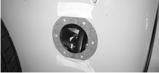
Fig 16 Gasket positioned on back panel
