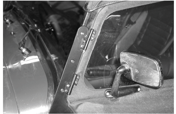
Fig 4 Hinge and sidescreen fitting
