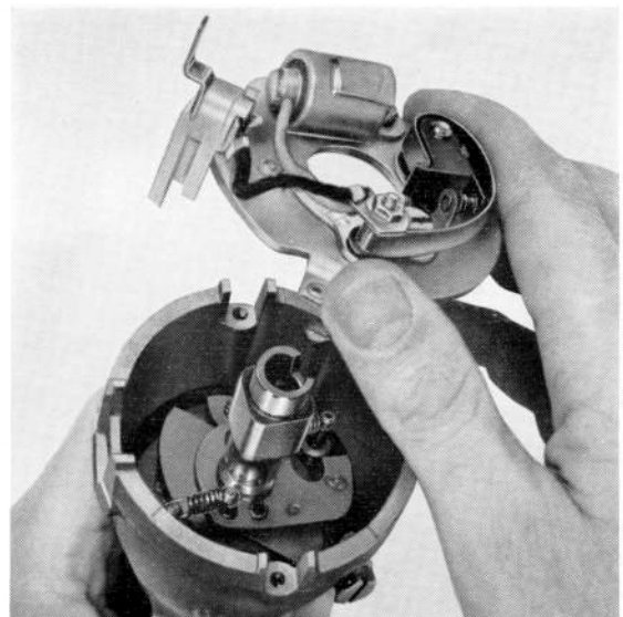
Replacing the Breaker Plate Assembly
