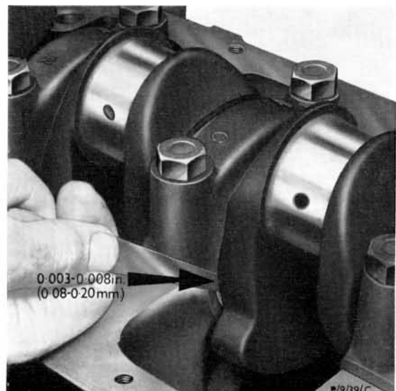
Checking the Crankshaft End-float
