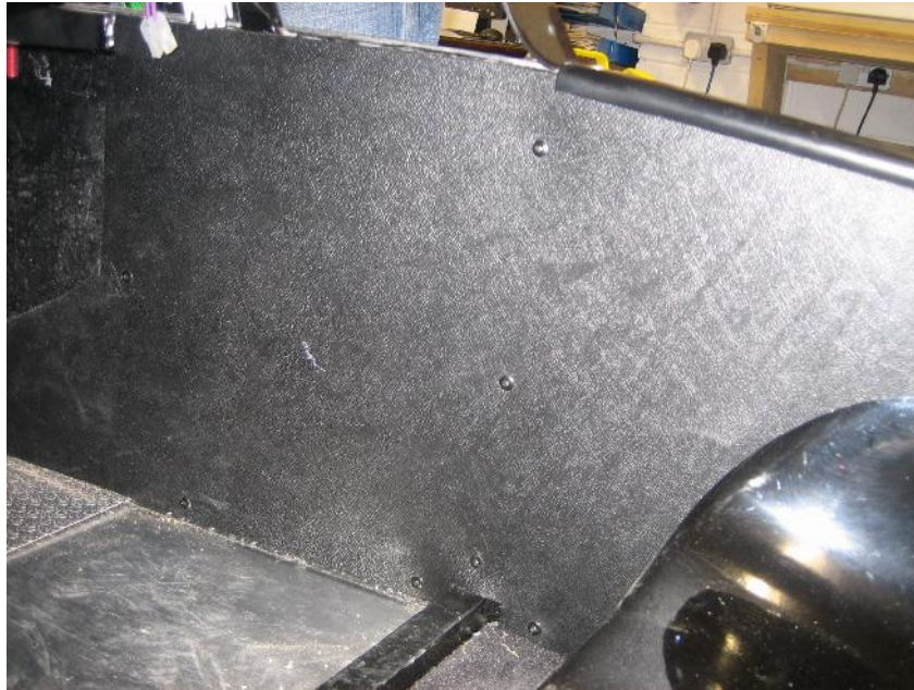
Internal panel fitted to side.
