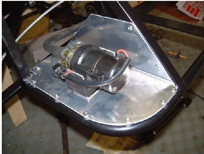
Car Fuel pump mounted
