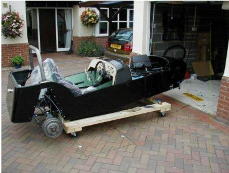
External panels fitted
