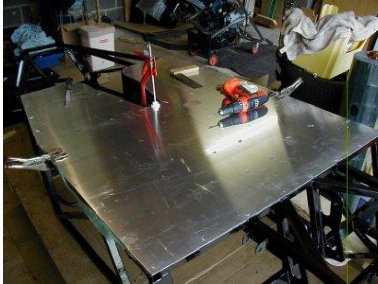
Pop riveting the floor.
