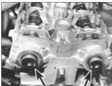
11.34 Camshaft roll pin locations at TDC position for refitting camshaft carrier (arrowed) - K16 engine
