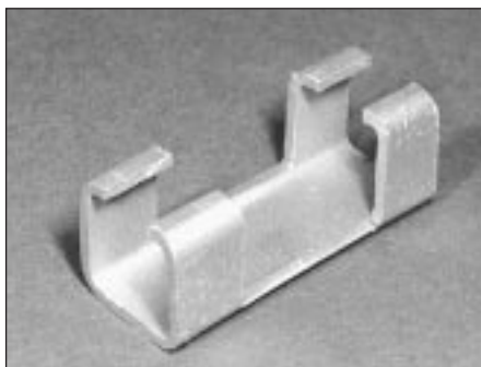
9.11a Camshaft locking tool cut from steel section . . .
