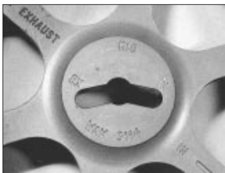
9.22 Camshaft sprockets have two keyways. Engage EX keyway with exhaust camshaft roll pin and IN keyway with inlet camshaft roll pin - K16 engine
