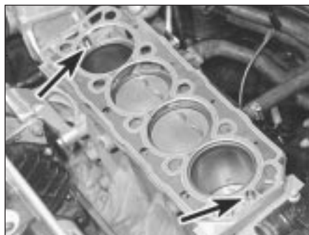
13.26a Fit new cylinder head gasket on two locating dowels (arrowed) . . .
