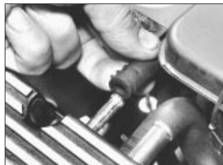
5.3b Disconnecting breather hoses from cylinder head cover - K16 engine
