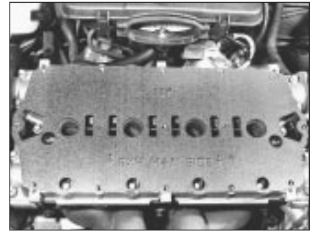
5.20b . . . stamped markings would appear as shown if gasket were placed on camshaft carrier
