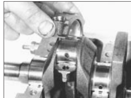
10.9 Removing No 1 cylinder big-end bearing cap and lower bearing shell
