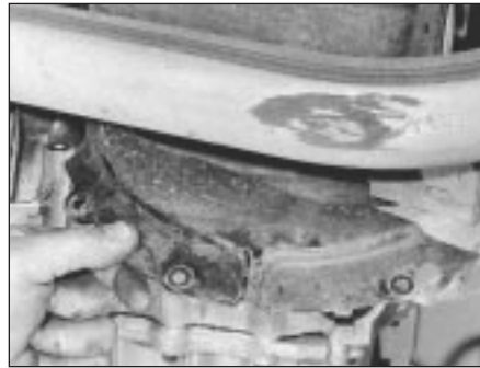
14.6 Remove flywheel lower cover plate to reach sump bolts
