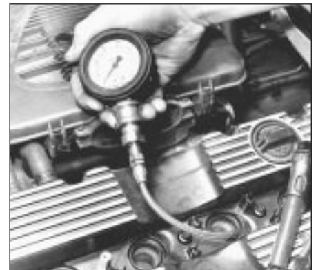
3.4 Measuring compression pressure
