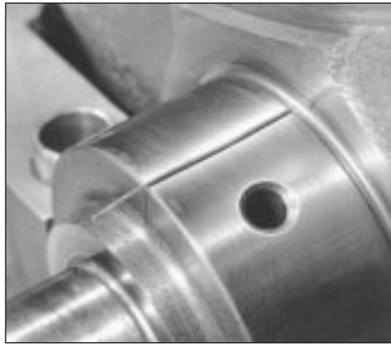
18.14 Lay length of Plastigauge on journal to be measured, parallel to crankshaft centre-line
