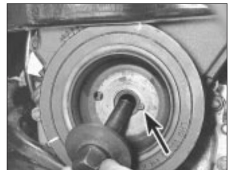
6.7 Ensure notch in crankshaft pulley centre fits over crankshaft timing belt sprocket locating lug (arrowed)
