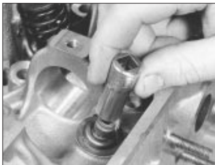
8.2 Using a socket to install valve stem seal
