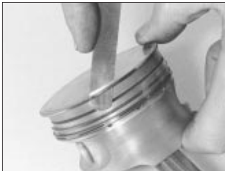
13.3 Removing piston rings with feeler blades
