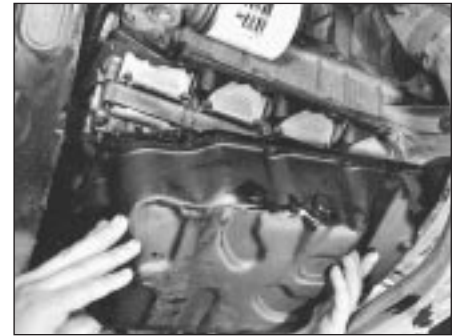
14.9 Removing the sump
