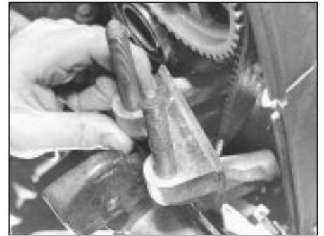
8.11 Removing engine/gearbox unit right-hand mounting bracket - K8 engine
