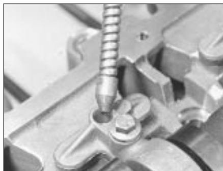
11.30a Fill oil holes with clean engine oil - K8 engine
