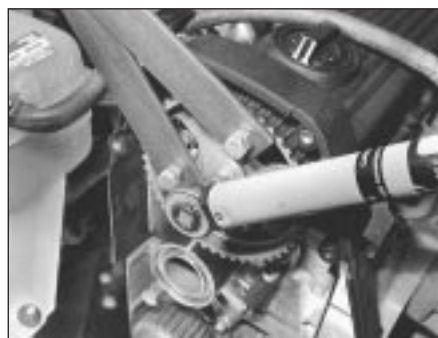
9.23a Using fabricated tool to hold camshaft pulley in position - K8 engine
