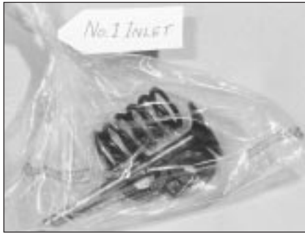
6.5 Use a labelled plastic bag to keep together and identify valve components
