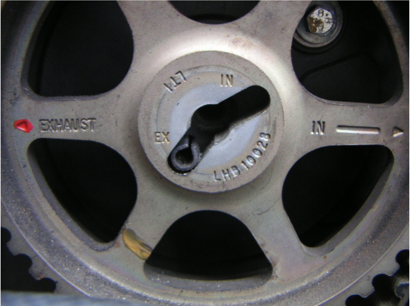
LHB10028 - EXHAUST PULLEY with its locking bolt removed to show that the slot marked 'EX' must be located over the roll pin.
