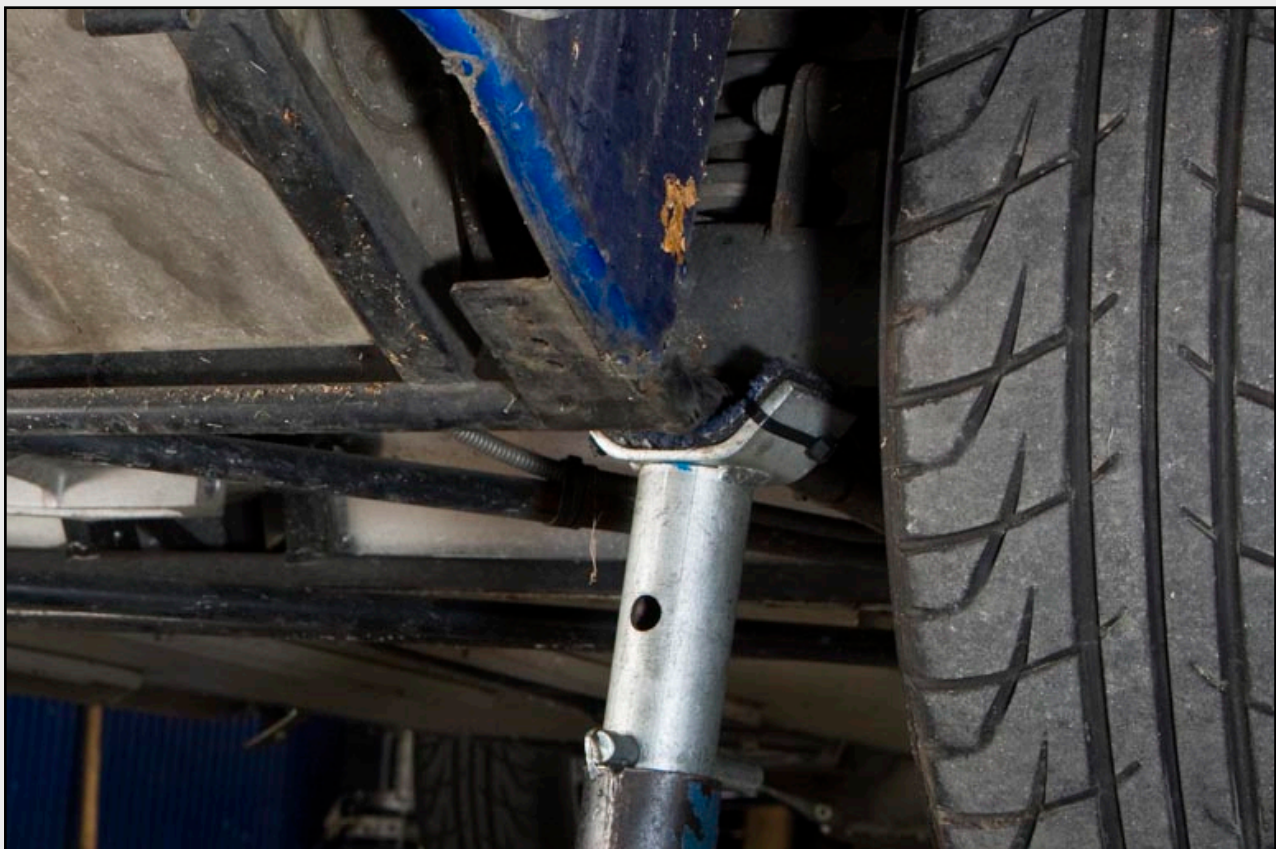
Fig 2a Close Up: axle stand supporting rear of S3 or SV (right-hand side), just ahead of the fuel tank
