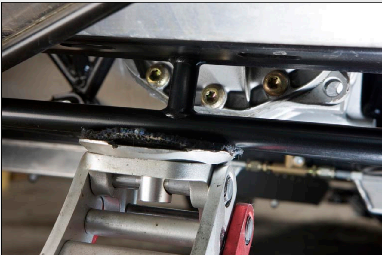
Fig 1b Close Up: of the CSR jacking position at rear with the saddle of jack under centre of chassis
