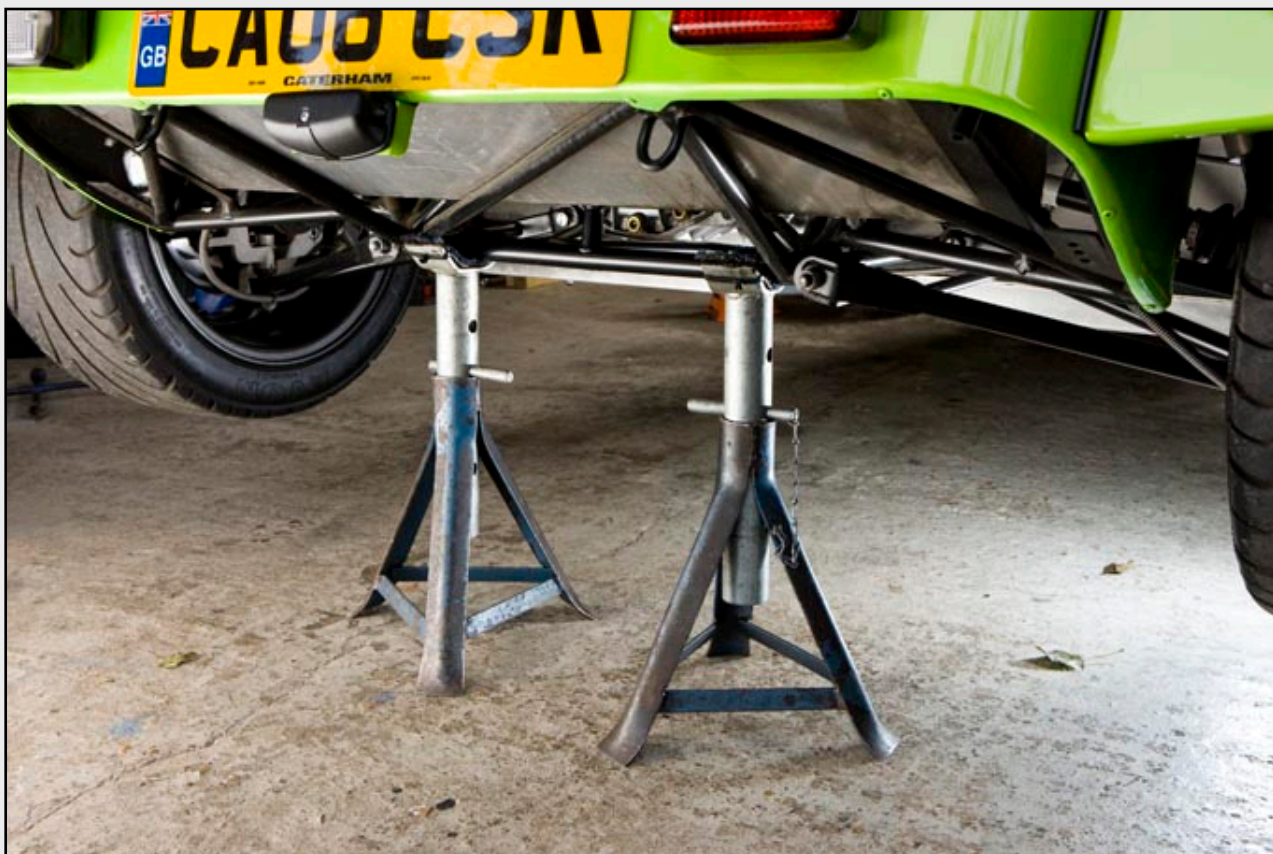
Fig 2b: CSR axle stands at rear when the jack has been removed
