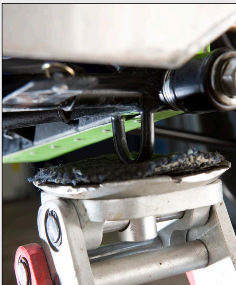
Left: The jack positioned under towing eye at front of CSR
