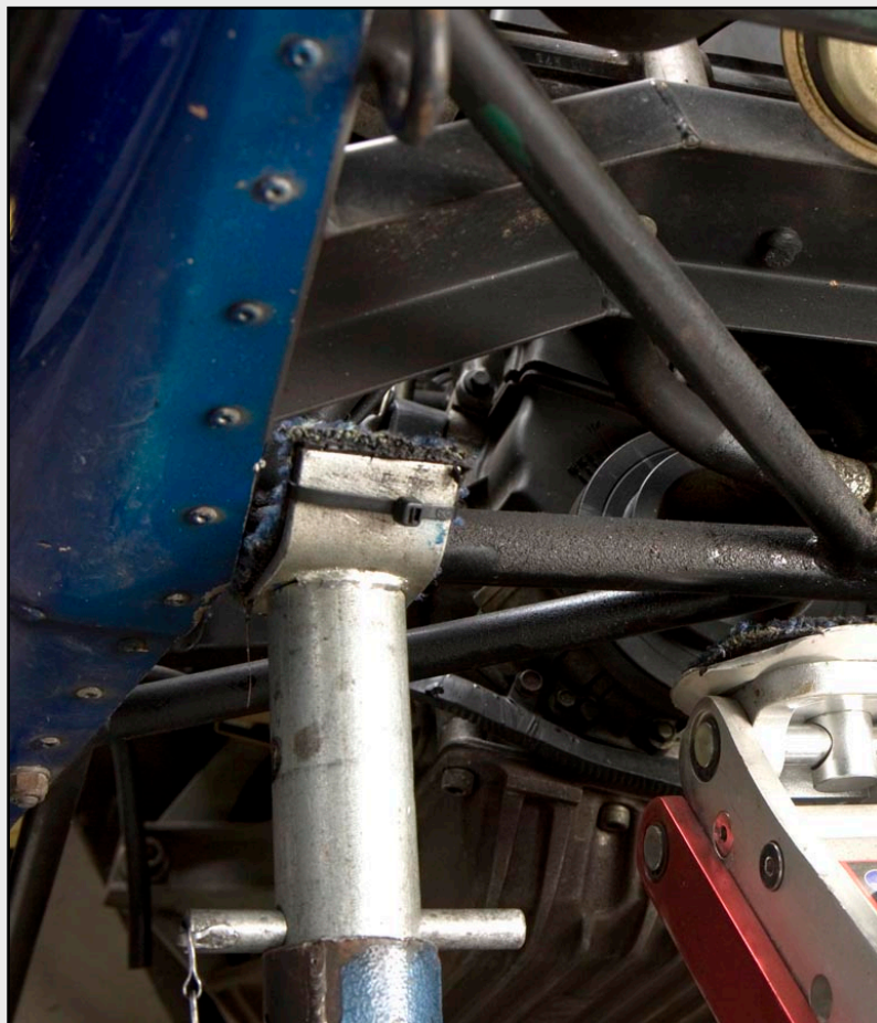
Left: The square of carpet or other padding fixed to top of axle stand
