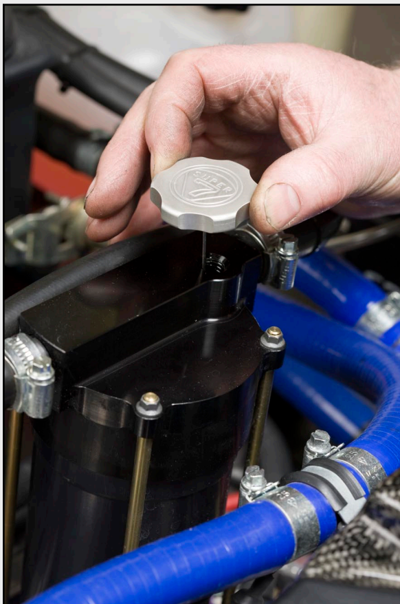
Figs 4&5: CSR, dipstick fitting in the dry sump system swirl-tower
