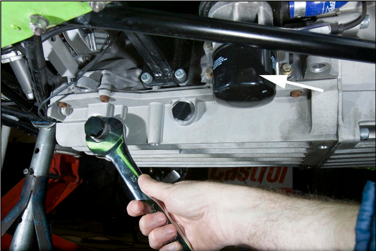
Fig 3: CSR, using a spanner on the drain plug of the dry sump pan; a gauze filter is behind this plug; (main oil filter is arrowed)
