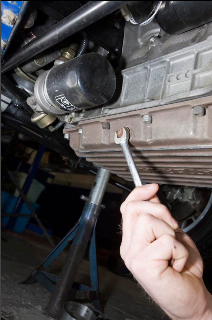
Fig 6: ( left ) S3 or SV, K-series engine, loosening the drain plug for the sump pan (left-hand side of car; oil filter is the black can above it)
