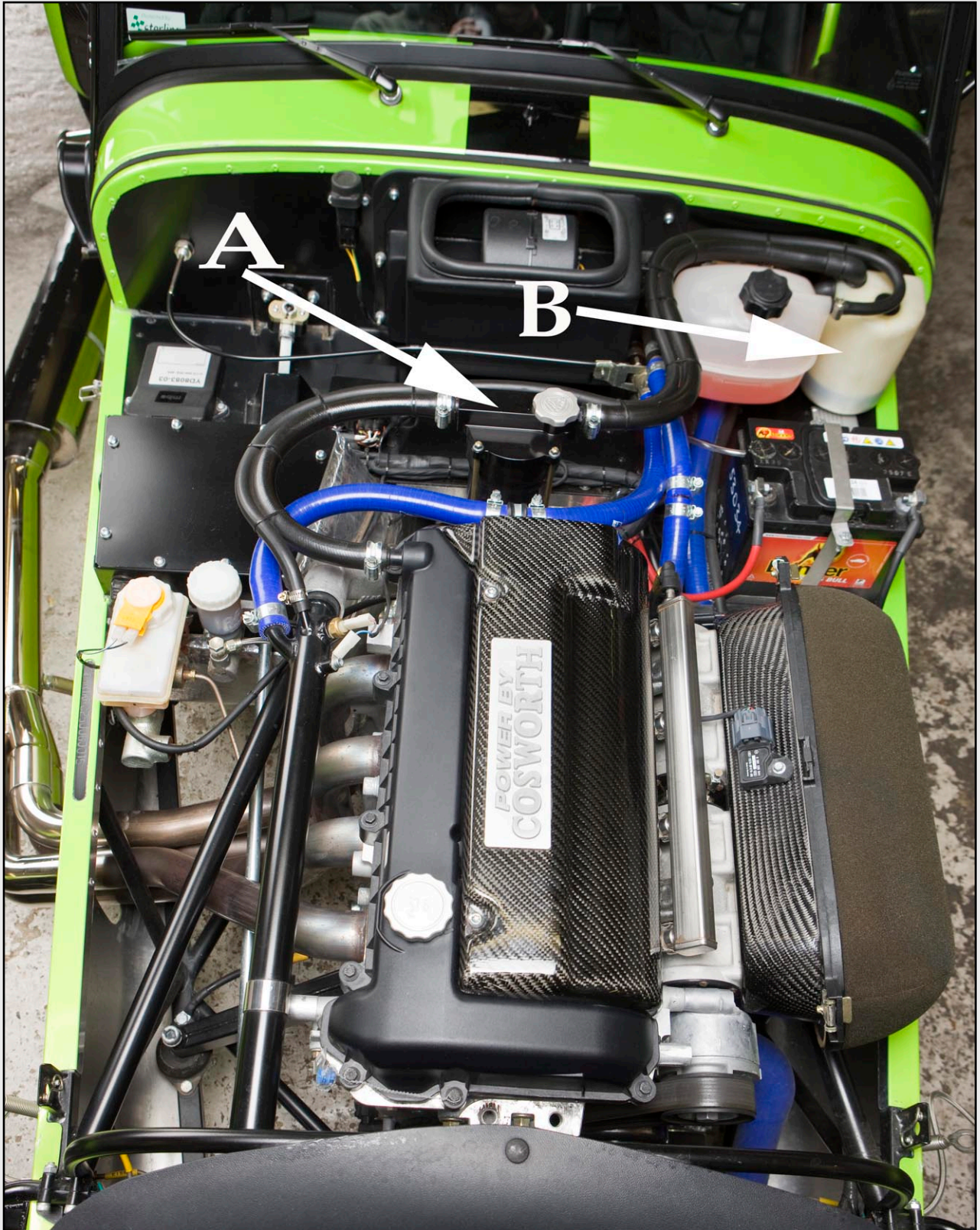
Fig 1: CSR engine bay; items referred to in the text include the black swirl-tower (arrowed A) for the dry-sump oil system on the centre-line of the car, behind the cylinder head, and the catch-tank on the near side edge of the scuttle. Right, (arrowed B).
