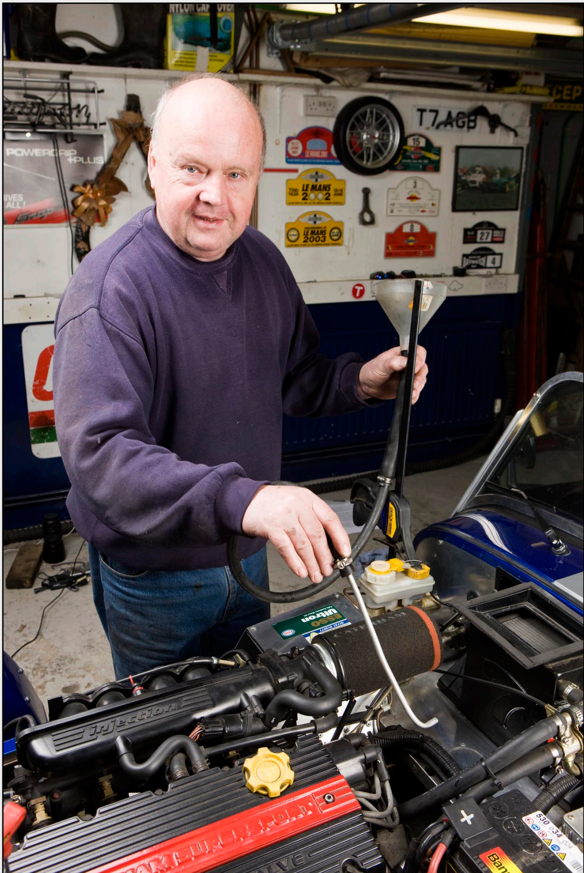
Fig 4: An improvised devise for replenishing gearbox or diff oil: funnel, hose and angled pipe for oil delivery (see text).
