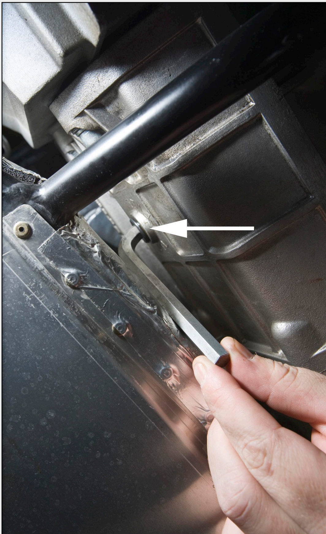
Fig 3 (Above): A view from beneath car showing oil filler/level plug on side of 6-speed 'box (in this case in CSR chassis) with Allen key in place in the plug. In both cases the front the car is at the top of the picture.
