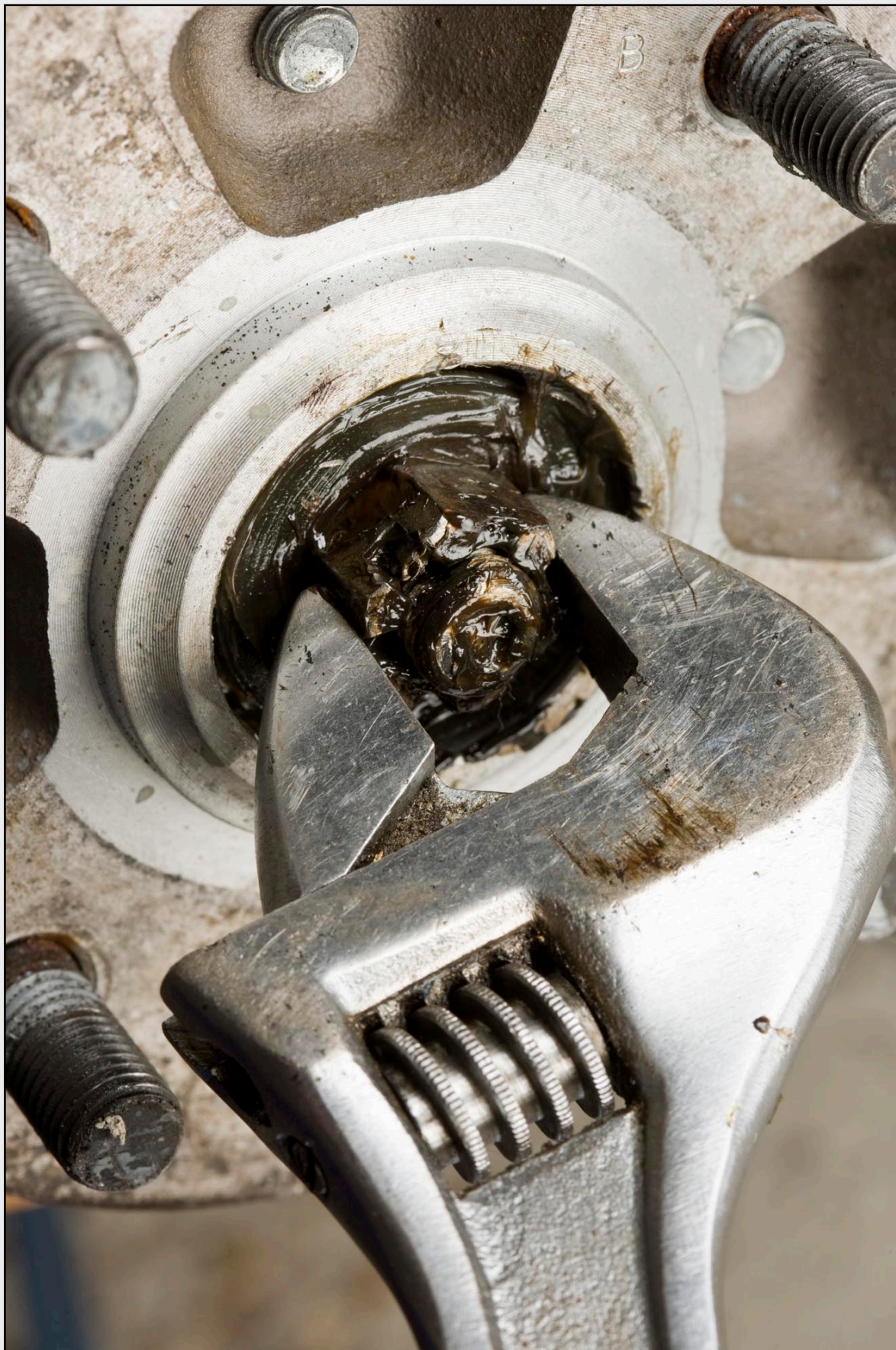
Figs 5: The castellated nut can be turned, with a large spanner or socket, to remove it or to adjust the bearing (see text).
