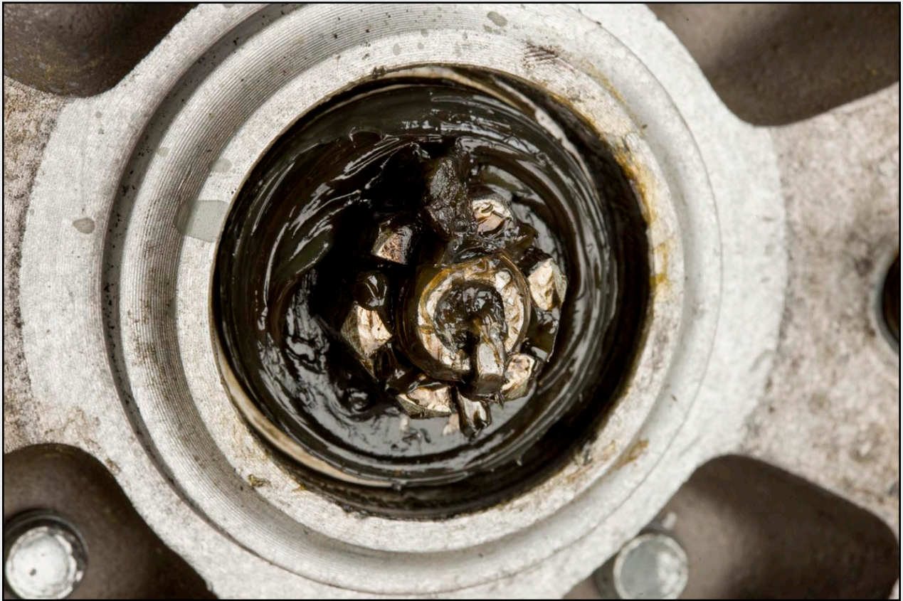
Figs 3: Visible amid the grease of this well-packed bearing are the end of the stub axle with the castellated nut and split pin through them.
