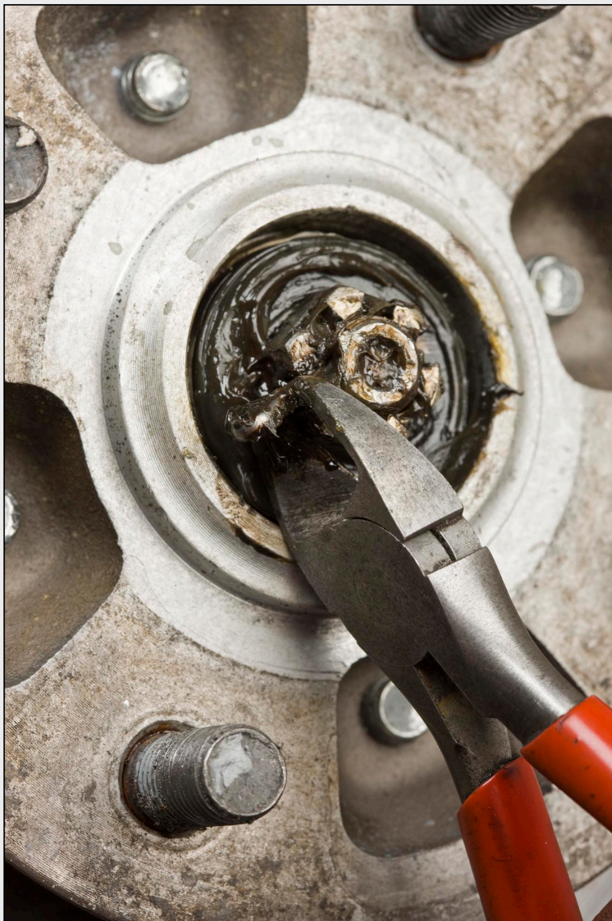
Fig 4: With its 'legs' straightened, the split pin can be pulled from the nut and stub axle. Replace the split pin, don't re-use the old one.
