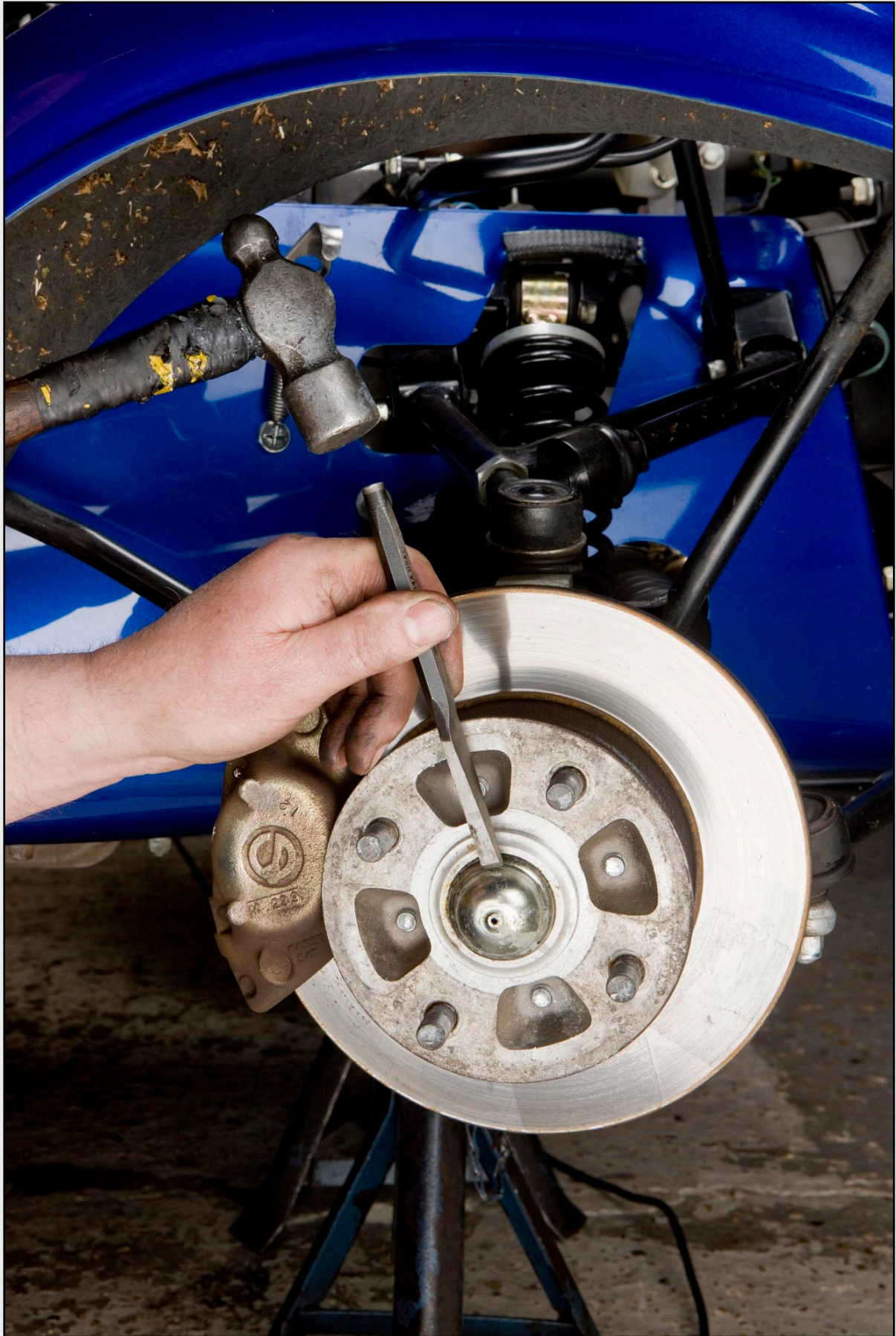
Figs 1 (Above) and 2 (Next Page): Removing the dust cap from the hub.
