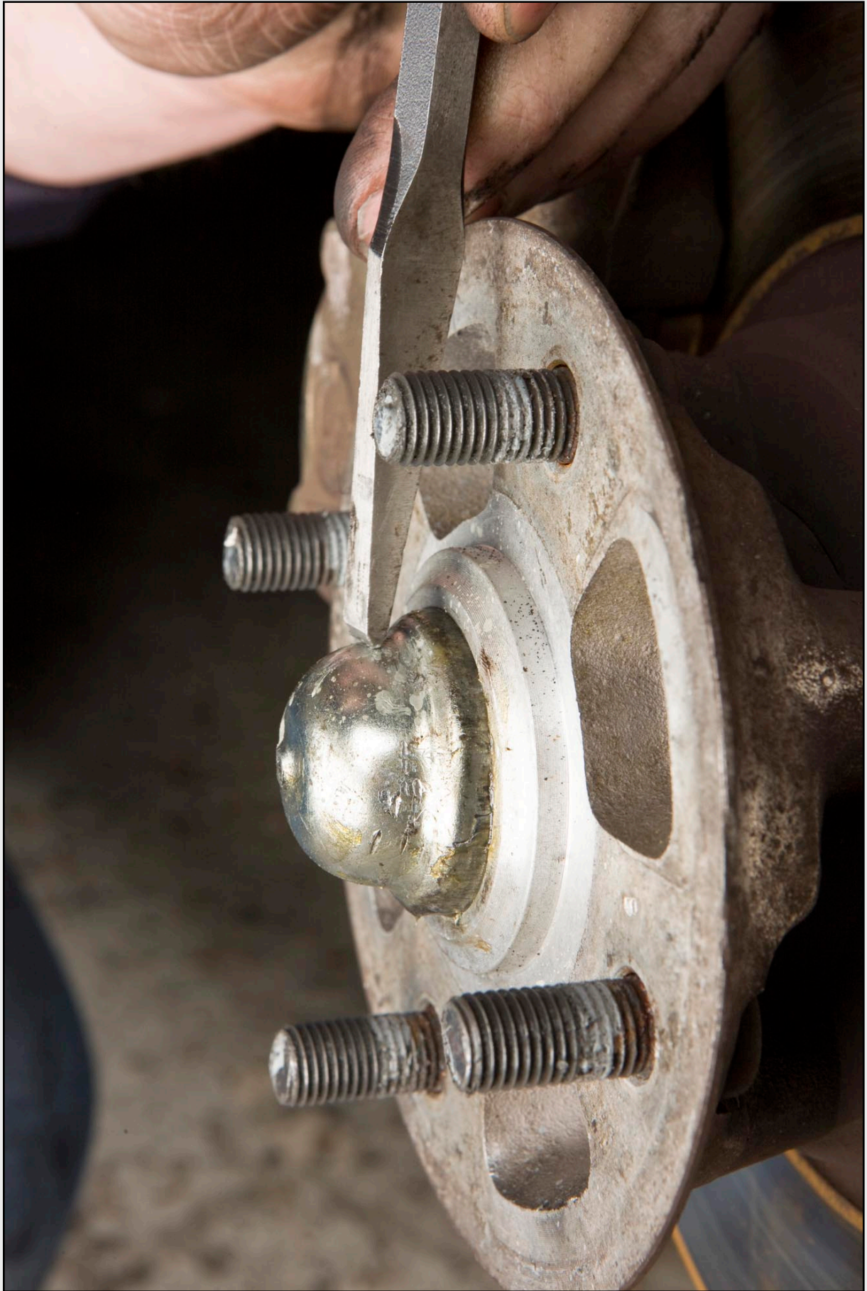
Figs 1 (Previous Page) and 2 (Above): Removing the dust cap from the hub.
