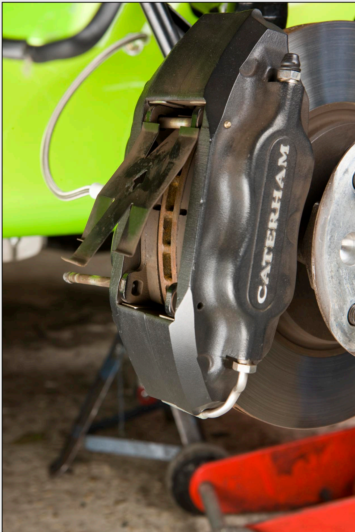
Fig 5: with the retaining pins removed, the shields can be sprung out...
