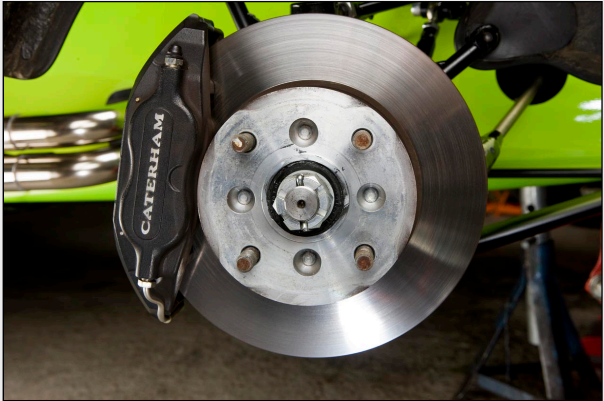
Front right-hand hub, brake disc and four-piston caliper, seen here on a CSR model.
