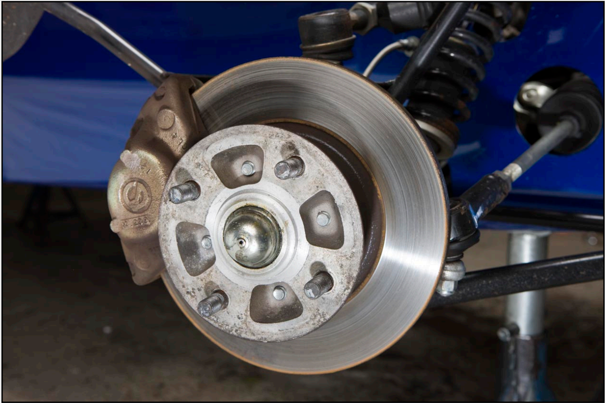
Front right-hand hub, brake disc and two-piston caliper: the typical standard 'S3' Caterham set-up.
