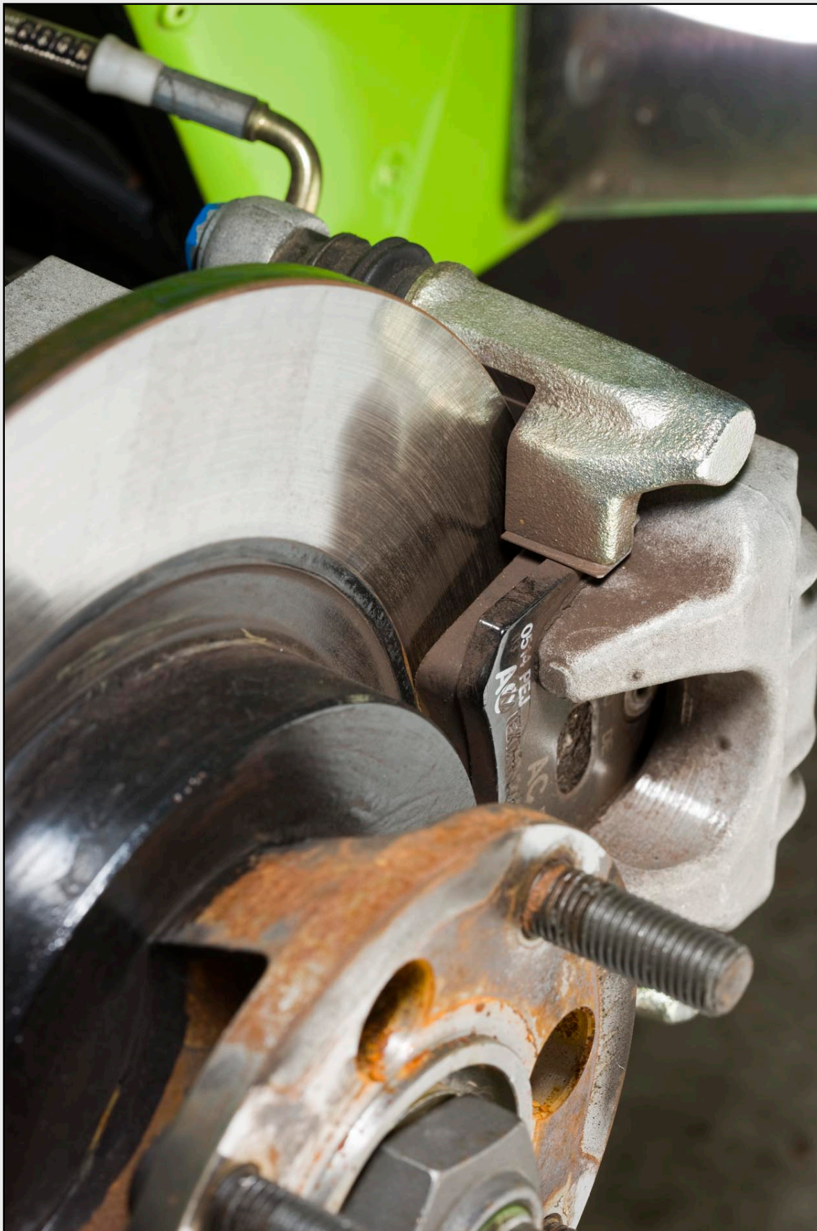
Fig 7: ... single-piston rear caliper; this is the right hand side and the outer brake pad is arrowed.
