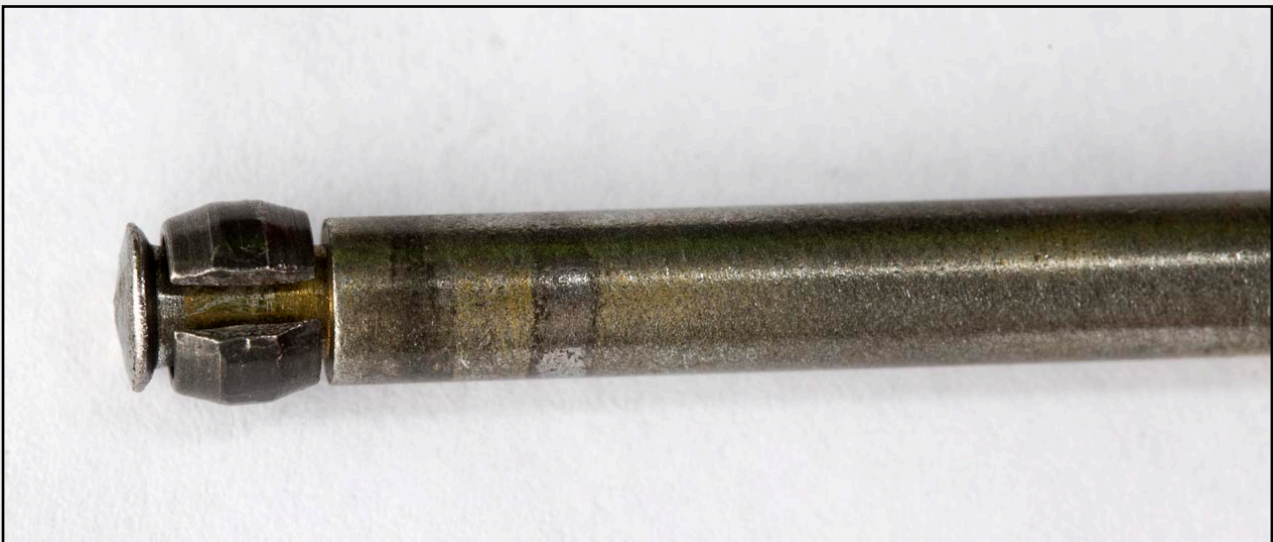
Fig 4: each pin has a retaining clip (see text).
