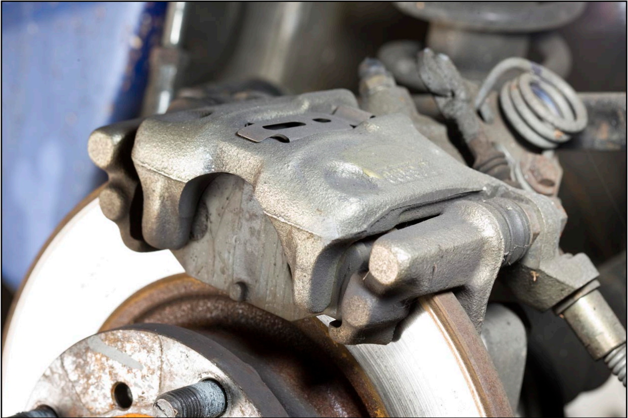
Fig 11: the standard single-piston, 'Ford Sierra-type' caliper used at the rear grips the brake disc at the top; this the right-hand side. (The coiled spring at top right and the cable running forward are for hand brake actuation.)
