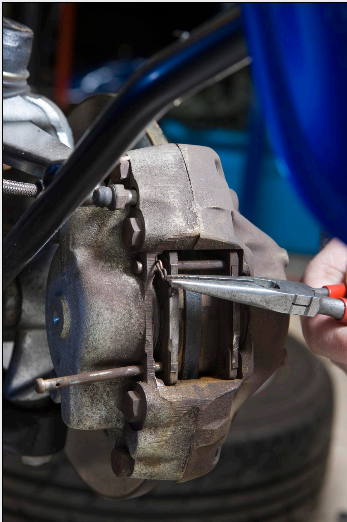
Fig 9: removing the 'R' clips from the pad-retaining pins and sliding the pins from the caliper.
