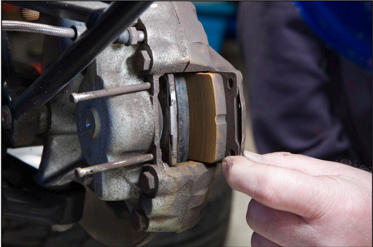
Fig 10 , top: withdrawing the pads from the back of the caliper. Note the pads here have a thin metal shim slotted between pad and piston; sometimes called an 'anti-squeal shims', they also stop the pads rattling (note how these fit before you pull them out).
