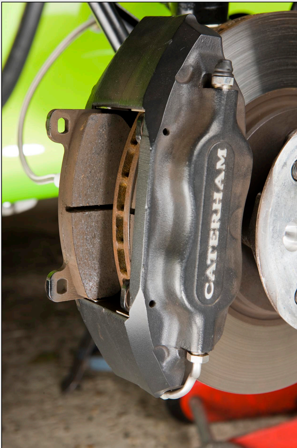
Fig 6: ...and the brake pads pulled out from the back of the caliper.
