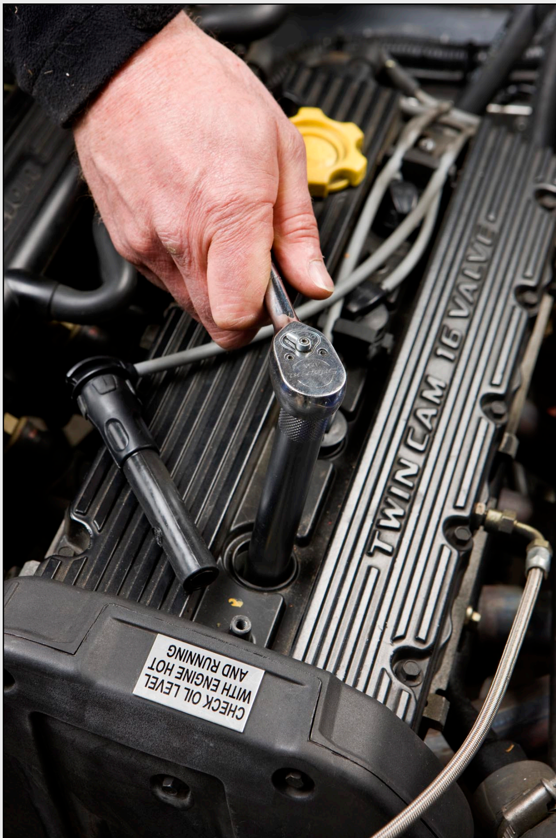
Figs 5, with the plug cover removed, the leads can be pulled off and the plugs then removed with the long-reach socket.
