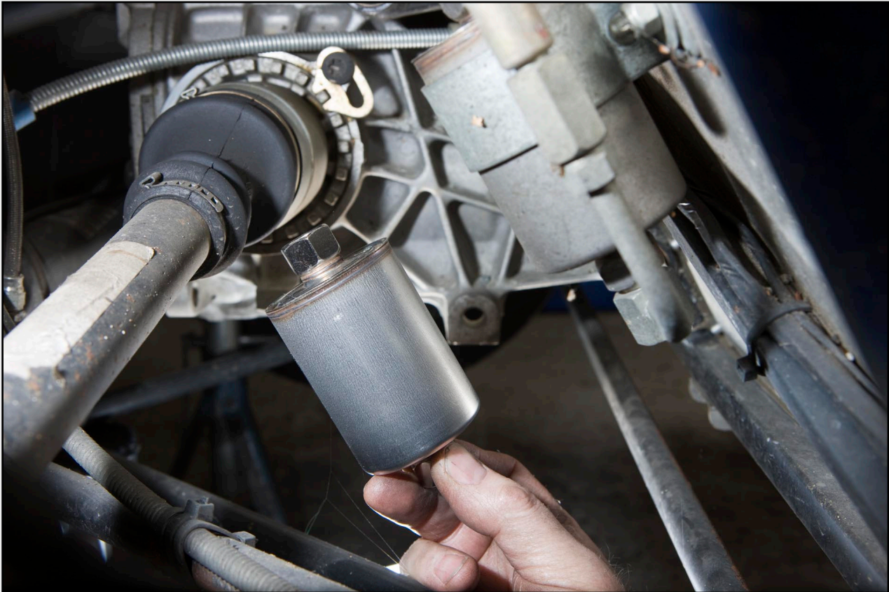
Fig 3 Previous Page and 4 Above: the fuel filter (arrowed)... this is the typical installation for a Rover K-series engined car, mounted on the back of the cockpit bulkhead behind the seats... ...and this is the canister of the filter removed from car. If you are confused by this view, we are looking through the right rear wheel arch, ahead of the brake disc.
