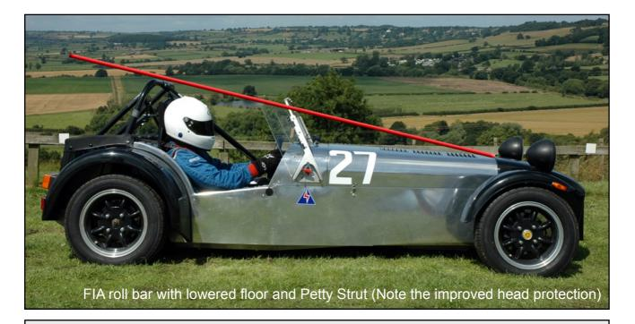
**Petty Strut:** In these pictures the 'Petty Strut' is fitted to the FIA roll bar. It can be seen located just behind the driver and is fitted to the top central area of the FIA roll bar with the other end fitted to the car's chassis on the passenger's side of the transmission tunnel in the foot well. This gives the FIA roll bar much greater strength through improved points of triangulation support in the rigidity of the safety device.
