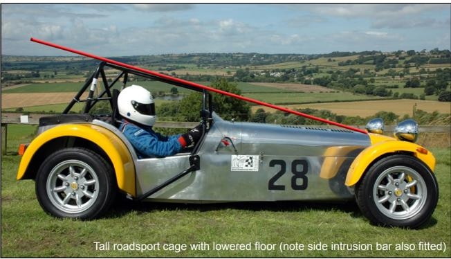
**Roadsport cage:** Further tubes run from the top or the roll bar forward to a point near the top corners of the windscreen and down to the dash panel to form a complete cage. This gives the occupants even more protection but makes the car more difficult to get into, windscreen and weather protection can still be used although erecting the hood is a little more difficult than with a roll bar. *More track orientated than road.*
